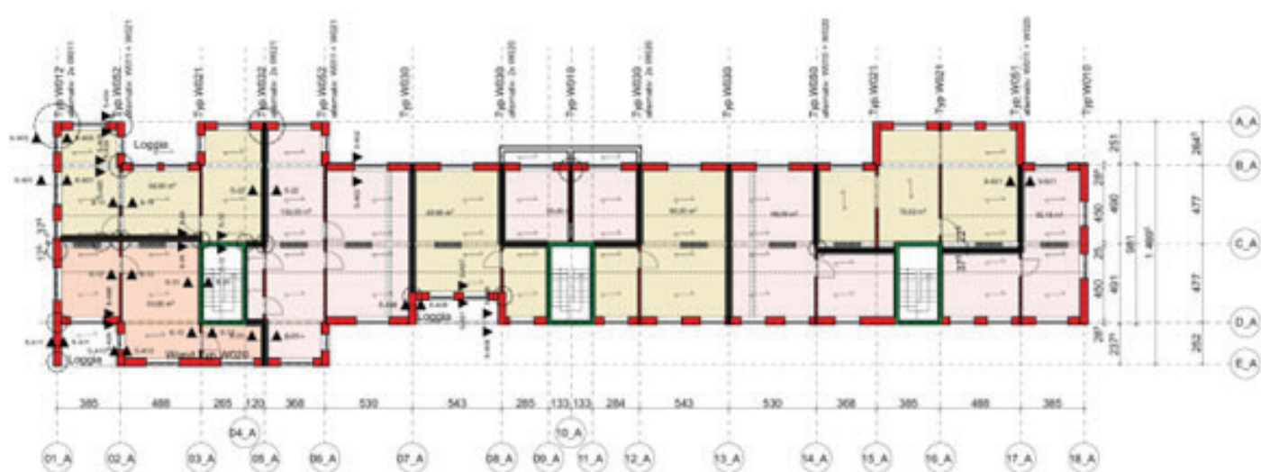
Figure 1: Representative floor plan with planned addition of stories, based on 33 real buildings
