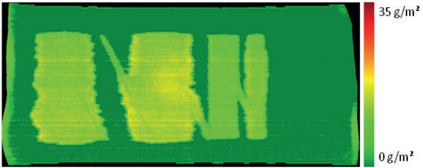
Figure 1. Spectral image of polyester fabric which was locally finished with a colorless flame retardant by Chromojet printing.
