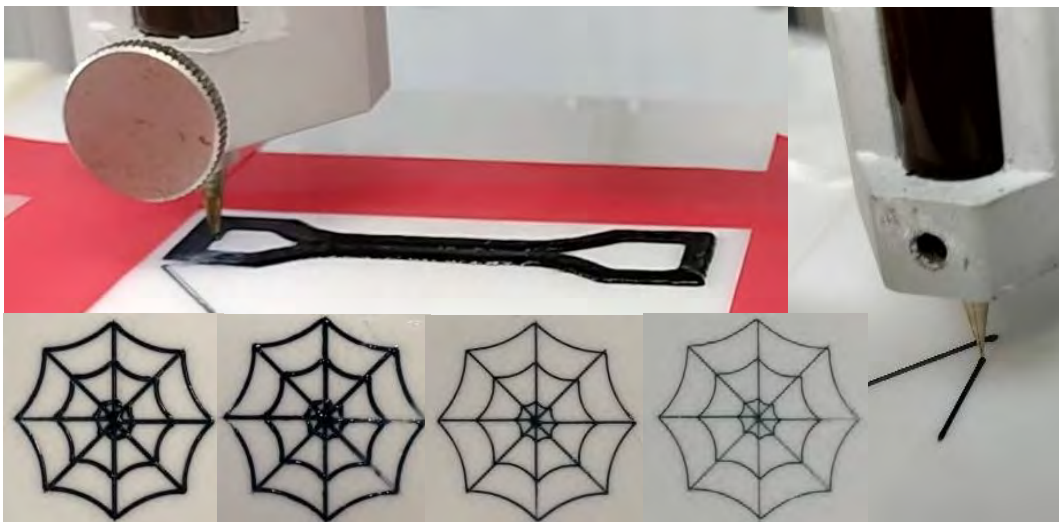
Figure 1. The top and right image show different structures being 3D printed with using conductive hydrogel material. The versatility of 3D printing allows for rapid iteration. The spider web structures are all printed with increasing amounts of methylcellulose from left to right, which increases the ink's viscosity and improves the resolution of the printed material. To an extent, this parameter can be optimized without influencing conductivity.
